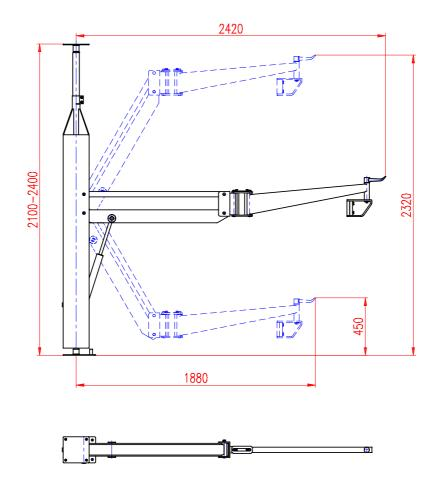
Manipulator is used as the additional attachment placed in the box of refrigerating truck. It enables the easy re-hanging of the pork halves and beef quarters from the aerial trail of the refrigerating truck to the customer aerial trail. Manipulator drive is hydraulic, aggregate is car electricity powered.
